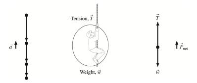
**Assess:** Note that the upward force from the rope must be greater than the downward weight force in order for the acceleration to be upward.
