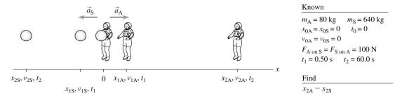
**SOLVE:** The astronaut and the satellite accelerate in opposite directions for 0.50 s. The force on the satellite and the force on the astronaut are an action/reaction pair, so both have a magnitude of 100 N. Newton's second law for the satellite along the *x*-direction gives
