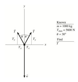
**SOLVE:** The beam attached to the ropes will remain in static equilibrium only if  $T < T_{\text{max}}$ , where  $T_{\text{max}}$  is the maximum sustained tension. The equilibrium equations in vector and component form are as follows:
