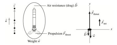
SOLVE: A force-identification diagram, a motion diagram, and a free-body diagram are shown.
