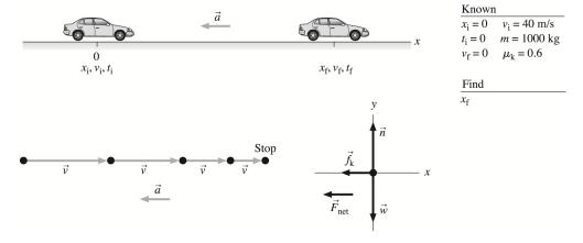
**SOLVE:** We begin with Newton's second law. Although the motion is one-dimensional, we need to consider forces in both the x- and y-directions. However, we know that  $a_y = 0$  m/s<sup>2</sup>. We have
