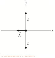
**SOLVE:** Since the locomotive does not accelerate in the vertical direction, the free-body diagram shows that n = w = mg. The friction force is  $f_r = \mu_r mg$ .
