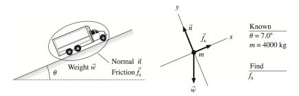
ASSESS: The truck's weight (mg) is roughly 40,000 N. A friction force that is  $\approx 12\%$  of the truck's weight seems reasonable.
