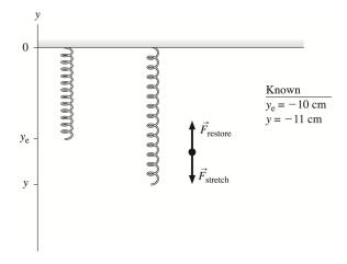
**SOLVE:** (a) The spring force or the restoring force is  $F_{\rm sp} = -k\Delta y$ . For  $\Delta y = -1.0$  cm and the force in Newtons,
