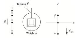
**ASSESS:** Note that if the elevator had been moving downward at a constant speed, the tension would need to be the same magnitude as the weight. Only because the elevator is speeding up as it descends, we know the net force must be downward.
