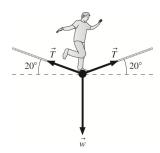
**SOLVE:** The only forces on the piece of rope under the student's foot are the two tension forces and the downward weight of the student.
