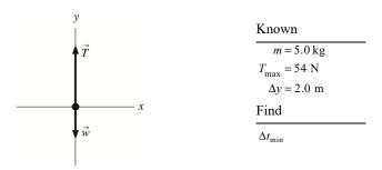
**SOLVE:** Since we want the shortest possible time, we'll use the maximum tension, which produces the maximum acceleration.
