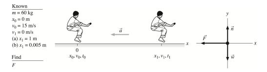
**SOLVE:** (a) In order to use Newton's second law for the passenger, we'll need the acceleration. Since we don't have the stopping time,
