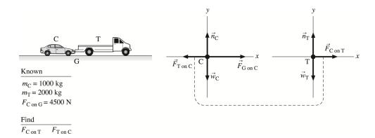
**SOLVE:** (a) The x-component of Newton's second law for the car is
