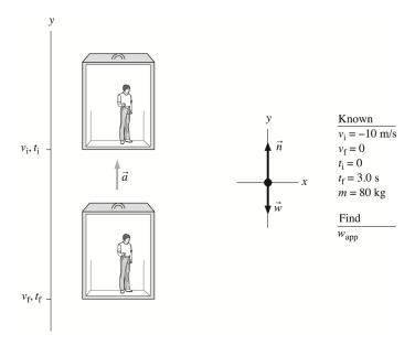
SOLVE: (a) Before the elevator starts braking, Zach is not accelerating. His apparent weight is
