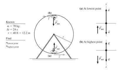
A preliminary calculation gives the speed:  $v = \frac{2\pi r}{\Delta t} = \frac{2\pi (12.2 \text{ m})}{24 \text{ s}} = 3.19 \text{ m/s}$
