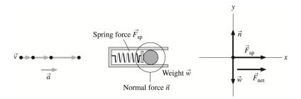
ASSESS: Since the normal force acting on the ball and the weight of the ball are equal in magnitude and opposite in direction, the ball experiences no vertical motion.
