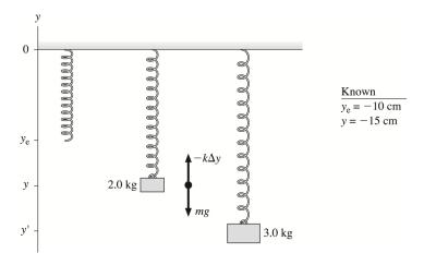
**SOLVE:** (a) The spring force on the 2.0 kg mass is  $F_{sp} = -k\Delta y$ . Notice that  $\Delta y$  is negative, so  $F_{sp}$  is positive. This force is equal to mg, because the 2.0 kg mass is at rest. We have  $-k\Delta y = mg$ . Solving for k:
