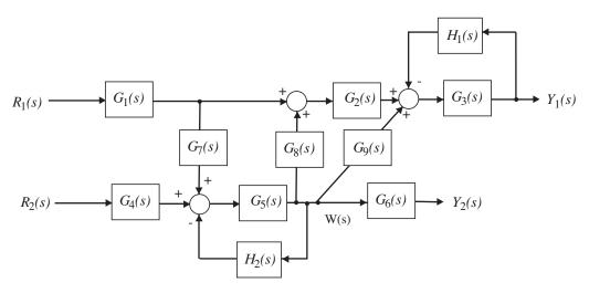
FIGURE E2.14 Block diagram model.
