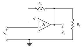
FIGURE E2.5 Noninverting op-amp circuit.
