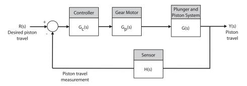
FIGURE E2.10 Shock absorber block diagram.
