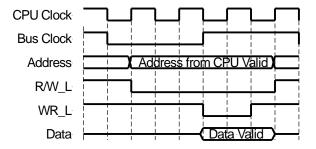
2.13 Draw a timing diagram relative to the system CPU clock shown in the figure below, which includes the address and data buses, R/W\_L, and the read control signal (RD\_L = active low) and which shows a read cycle. [a]
