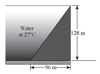
$\begin{aligned} & Width = 100m \\ & H_20@27^{\circ}\text{C} \quad \rho \text{=}997 \text{ kg/m}^3 \end{aligned}$
