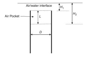
**2.6** Hydrometers are inexpensive and easy to use to measure specific gravity and then density. You want to measure the density of an unknown liquid, but all you have is a test tube that is 1 cm in diameter. You fill the test tube with water and drop it into a known sample of water with a temperature of 20C, and
