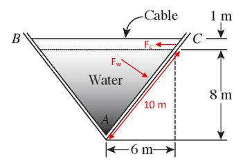
$$F_w = \rho_g g \overline{\bar{y}} A = (1000)(9.81)(4)(10)(1) = 392 \; kN$$
