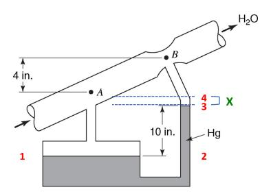
A differential manometer is used to measure the pressure change caused by a flow constriction in a piping system as shown. Determine the pressure difference between points A and B in psi. Which section has the higher pressure?
