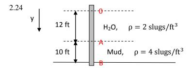
$$\begin{array}{l} P_{A}\text{-}P_{atm} \!\!=\!\! \rho_w g(12) \!\!=\!\! 24g \\ P_{B}\text{-}P_{atm} \!\!=\!\! 24g \!\!+\!\! 40g \!\!=\!\! 64g \end{array}$$
