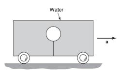
Pressure Gradient is in direction of  $\vec{g}$ - $\vec{a}$  & isobars are perpendicular to  $(\vec{g}$ - $\vec{a})$
