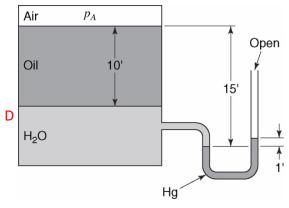
What is the pressure p<sub>A</sub> in the figure? The oil in the middle tank has a specific gravity of 0.8. Assume that the entire system is at 80°F.
