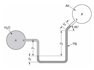
Referring to the figure at left, please find the pressure difference between tanks A and B if  $d_1$ =2 feet,  $d_2$ =6 inches,  $d_3$ =2.4 inches and  $d_4$ =4 inches.
