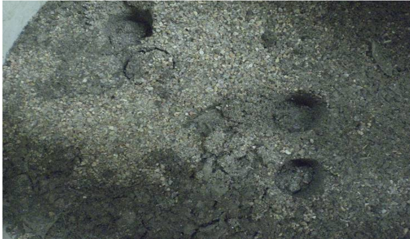
Surface Deposit (Cake Layer) after Long-term Infiltration Simulation with Sediment-laden Stormwater
