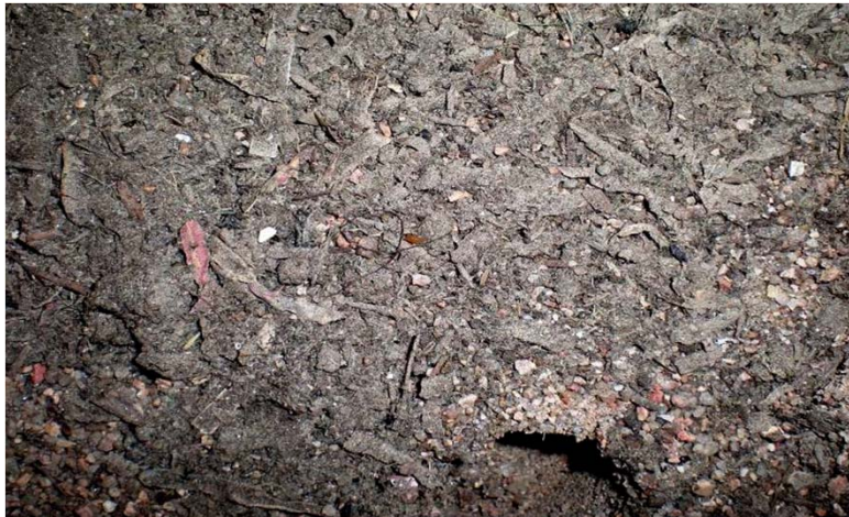
Surface Deposit (Cake Layer) after Long-term Infiltration Simulation with Sediment-laden Stormwater
