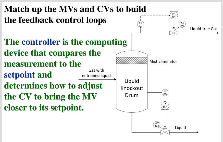
Match up the MVs and CVs to build the feedback control loops
