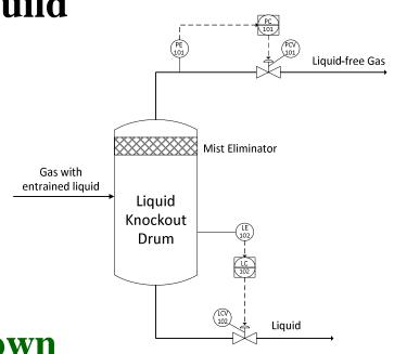
Match up the MVs and CVs to build the feedback control loops – match them up for best stability -- minimize interactions
