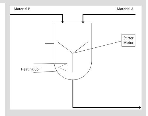
Once all of B has been consumed, additional component B is added to the reactor and the process is repeated until all of component A has been consumed. Now that the drum/tank contains virtually all component C, the fluid is drained out of the drum/tank.
