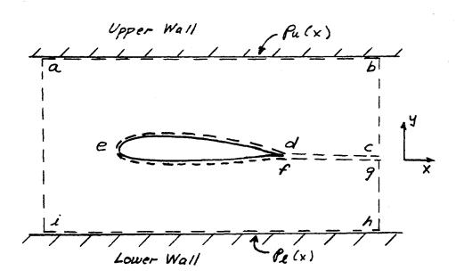
Denote the pressure distributions on the upper and lower walls by  $p_u(x)$  and  $p_\ell(x)$  respectively. The walls are close enough to the model such that  $p_u$  and  $p_\ell$  are not necessarily equal to  $p_\infty$ . Assume that faces  $\underline{ai}$  and  $\underline{bh}$  are far enough upstream and downstream of the model such that
