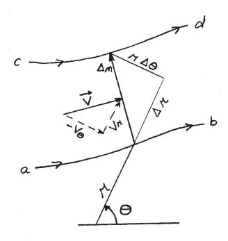
Mass flow between streamlines =  $\Delta \bar{\psi}$
