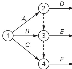
(a) The scheduling network is incorrect as shown in the text, because B precedes both D and E, while according to the problem it should only precede E. The correct network is obtained by introducing the dummy activity connecting events 3 and 4. Note that a dummy activity has zero duration.
