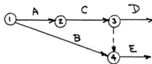
(b) The network in 4.10(b) is incorrect because as drawn A precedes D, E, and F while the problem states that A precedes only D and E. The correct network is
