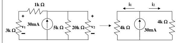
Using current division,  $i_1 = i_2 = (30 \text{ mA})(4 \text{ kohm}/(4 \text{ kohm} + 4 \text{ kohm})) = 15 \text{mA}$
