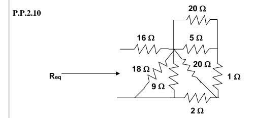
Combining the 9 ohm resistor and the 18 ohm resistor yields [9x18]/[9+18] = 6 ohms.
