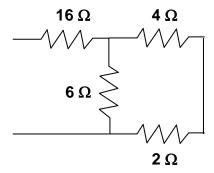
The 4 ohm and 2 ohm resistors are in series and can be replaced by a 6 ohm resistor. This gives a 6 ohm resistor in parallel with a 6 ohm resistor, [6x6/(6+6)] = 3 ohms. We now have a 3 ohm resistor in series with a 16 ohm resistor or 3 + 16 = 19 ohms. Therefore:
