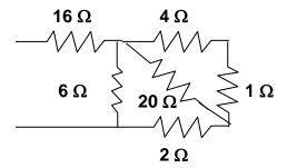
The 4 ohm and 1 ohm resistors can be combined into a 5 ohm resistor in parallel with a 20 ohm resistor. This will result in [5x20/(5+20)] = 4 ohms and the circuit shown below:
