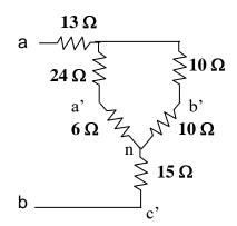
$$R_{a'n} = 20x30/[20 + 30 + 50] = 6 \text{ ohms}, R_{b'n} = 20x50/100 = 10 \text{ ohms}$$
