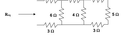
Combining the 4 ohm, 5 ohm, and 3 ohm resistors in series gives 4+3+5=12.
