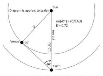
use the law of sines and the right triangle we have just created to solve for D. The right angle is at Venus when Venus appears to be farthest from the Sun (at greatest elongation). If the angle between Venus and the Sun is 46° as seen from Earth, then from trigonometry:
