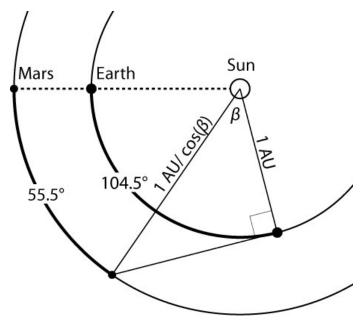
Using trigonometry it is possible to solve for the size of Mars's orbit more directly. The difference between the angles the two planets move is  $\beta = 104.5^{\circ} - 55.5^{\circ} = 49^{\circ}$  as shown in the diagram. The distance from the Sun to Mars is the hypotenuse of the right triangle, therefore
