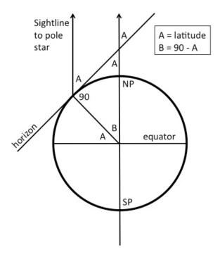
Note that this geometric demonstration makes use of several principles: a line (in this case the horizon) crossing parallel lines makes the same angle A to each, the sum of the angles in a triangle is 180°, and the tangent line to a point on a circle is at a 90° angle to the radius line to that point.
