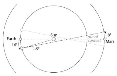
Mars's orbit 1.52 times larger than Earth's and ignoring the ellipticity.) By testing several angles with a protractor, shifting Earth by  $1^{\circ}$  per day and Mars  $\frac{1}{2^{\circ}}$  per day in their orbits around the Sun, it appears that Mars reaches an angle of  $\sim$ 5° from the Sun (as seen from Earth) about 16–18 days after conjunction. In total, then Mars is difficult to contact for about 32 to 36 days, counting the time before and after conjunction.
