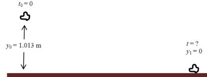
**RESEARCH:** For objects in free fall, equations 2.25 can be used to compute velocity and position. In particular, the equation  $y = y_0 + v_{y0}t - \frac{1}{2}gt^2$  can be used. In this case,  $y_0 = 1.013\,\mathrm{m}$ . Since the object is not thrown but dropped with no initial velocity,  $v_{y0} = 0\,\mathrm{m/s}$ , and  $g = 3.699\,\mathrm{m/s^2}$  on the surface of Mars.
