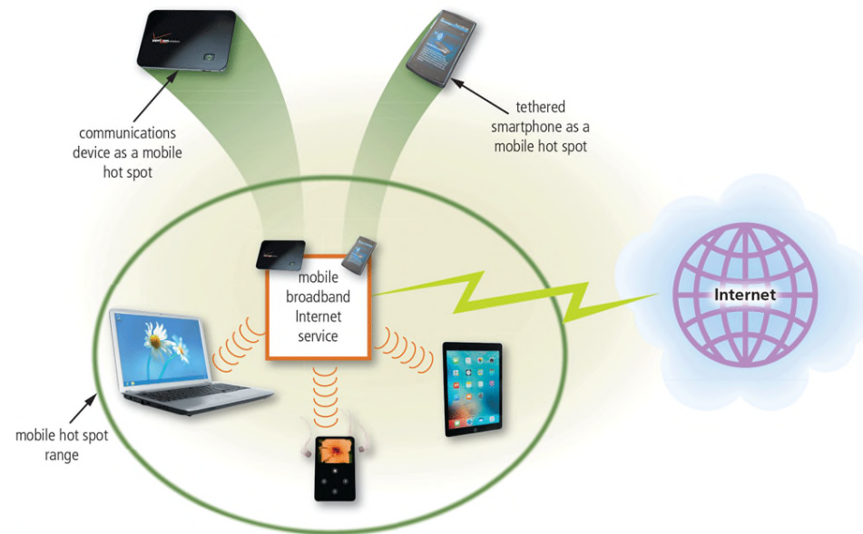
Figure 2-3 You can create a mobile hot spot using a communications device or by tethering a smartphone. Courtesy of Verizon Wireless; figarro / Can Stock Photo; iStockphoto.com / Mienny; amfoto / Shutterstock.com; Alex Staroseltsev / Shutterstock.com; Source: Microsoft
