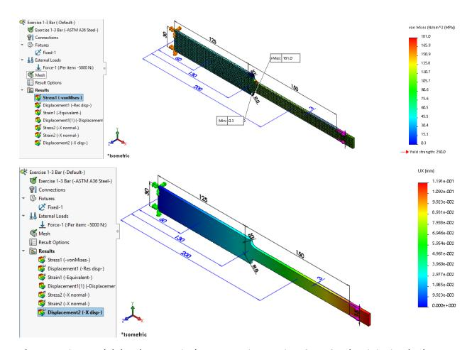
The 1D spring model development is the same as in Exercises 2.1 - 2.7, but it is simpler because it only has two springs, one for the 30-mm height bar section and the other for the 15-mm height section. Just modify the drawings and the MCAD worksheet for a two spring model.
