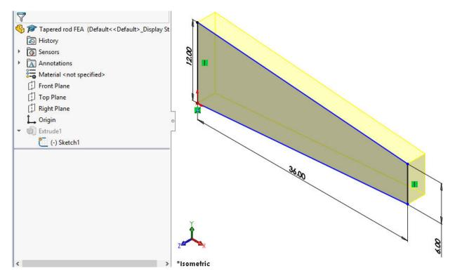
2.9. Refer to Exercise 2.1. Conduct an FEA and create a contour plot of the x-normal stress and displacement. Create and probe a section clipping at the nodes. Compare the FEA results with the spring-element model results. Explain any differences.
