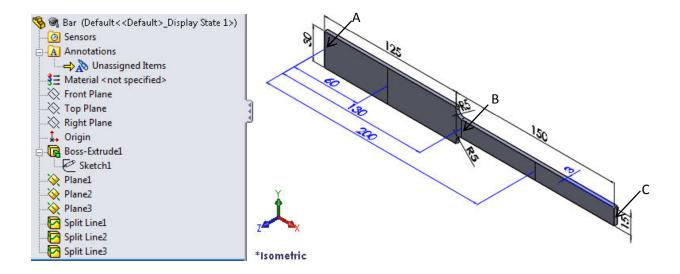
2.11. Create a 1D spring-element model for the 3D solid model from Exercise 2.10. Use ASTM A36 steel material, a fixed geometry restraint on the left-end face, a 5000 N load applied uniformly over the right-end face in the –y direction, and the default mesh. Create von Mises (vM) stress and x-displacement plots.
