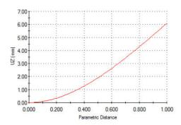
2.24. Refer to Exercises 2.16 and 2.23. To verify the FEA model configuration and to better understand the deformation probe plot shape and amplitude, use mechanics of materials fundamentals to create a graph of Uz(x) from B–B'. Compare with the FEA results probe plot and explain any differences. Compare the values of  $U_z$  @ x = 0 mm and  $U_z$  @ x = 1200 mm with the FEA results and the spring model and explain any differences.
