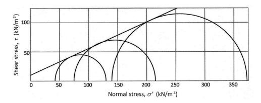
The failure envelope is drawn tangent to the Mohr circles in the figure and, from measurements,  $c' = 10.0 \text{ kN/m}^2$  and  $\phi' = 24.7^\circ$
